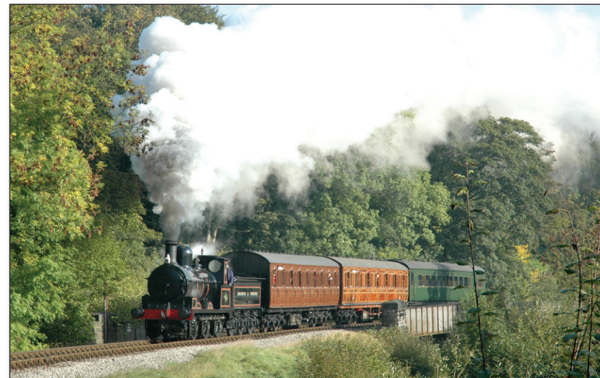
Perhaps best known as The Green Dragon in the EMI big screen production of Edith A Nesbit's classic The Railway Children , Lancashire & Yorkshire Railway Class 25 0-6-0 tender locomotive No 957 designed by Chief Mechanical Engineer William Barton Wright. Built by Beyer Peacock in Manchester, the type became known as 'Ironclads'.
